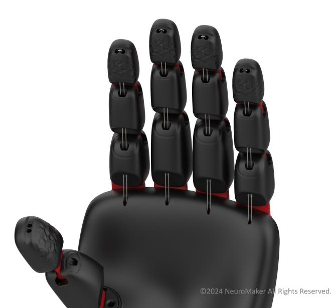
Repeat the previous steps to install tendon wires for the middle and index finger.
