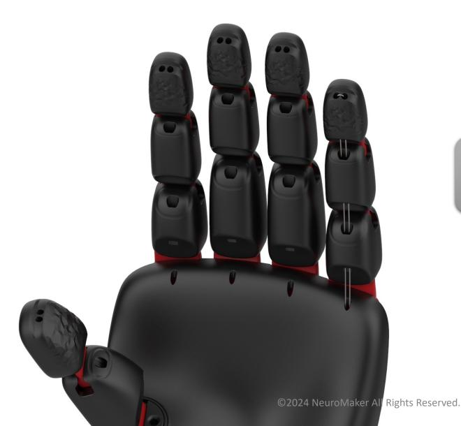
Pull the tendon wire downwards to tighten it, as shown in the illustration.
