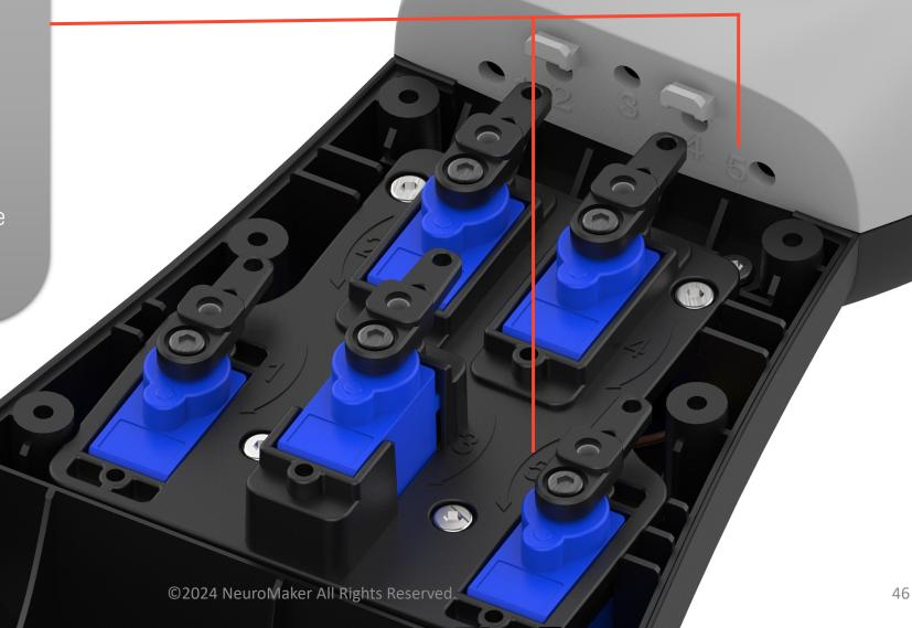
Step 1: Gently pull the tendon wires and thread them through the first hole of the servo arm, starting from the underside and guiding them upwards, through to the top side.
