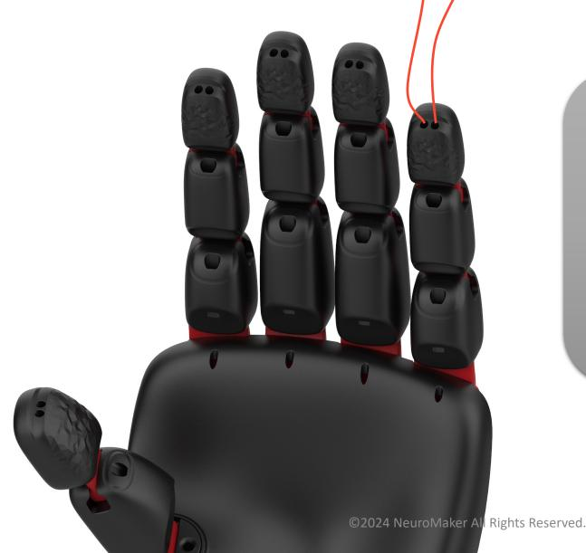
Step 1: Cut a piece of tendon wire with length equal to the span of your fully extended arms.
