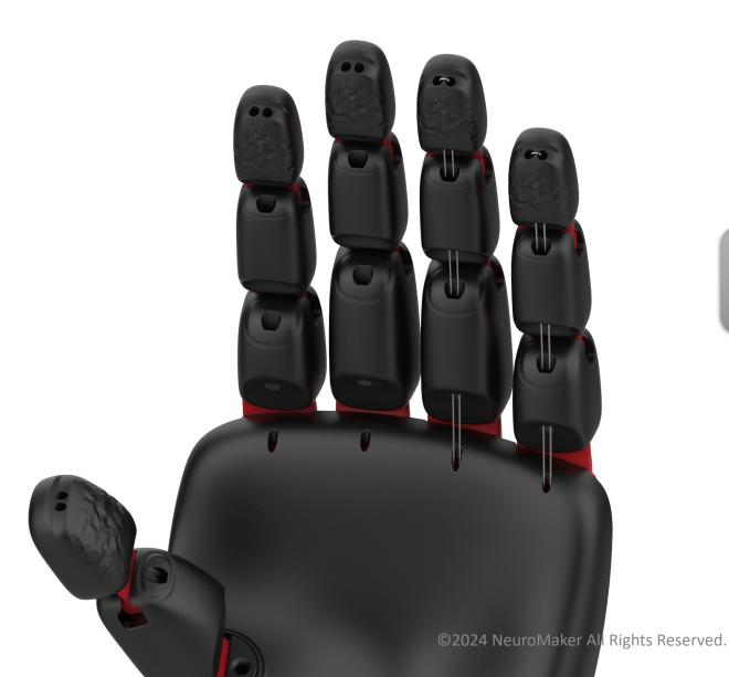
Repeat the previous steps to install a tendon wire for the ring finger.
